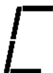
Flashing upper case C A call for second stage cooling has be received
