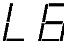
Active Protection – Code L6 – Compressor open start circuit
