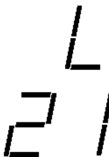
Active Protection – Code L21 – Open low pressure control
