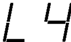
Active Protection – Code L4 – Locked rotor
