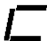
Flashing lower case c A call for first stage cooling has been received
